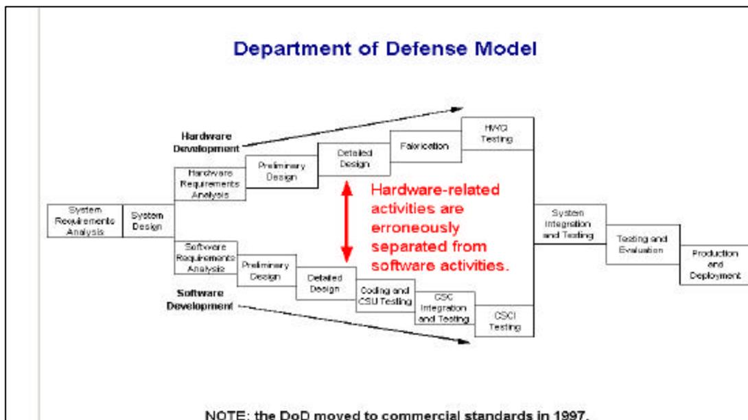
**Figure 6 - DoD Model for System Development [43]**
